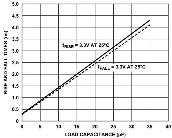
Figure 93. Driver Type A Typical Rise and Fall Times (10% to 90%) vs. Load Capacitance ( $V_{DD\_EXT} = 3.3 V$ )
