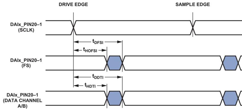
Figure 68. S/PDIF Receiver Internal Digital PLL Mode Timing
