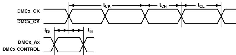
NOTE: CONTROL =  $\overline{DMC_x\_CS0}$ ,  $\overline{DMC_x\_CKE}$ ,  $\overline{DMC_x\_RAS}$ ,  $\overline{DMC_x\_CAS}$ , AND  $\overline{DMC_x\_WE}$ .
