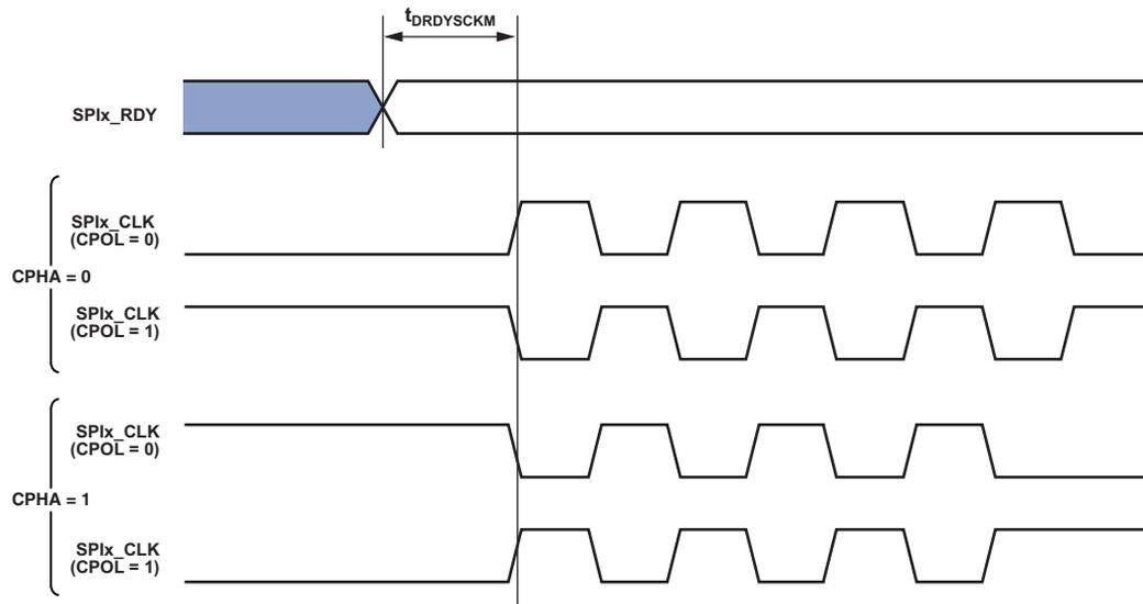
Figure 49. SPIx\_CLK Switching Diagram After SPIx\_RDY Assertion
