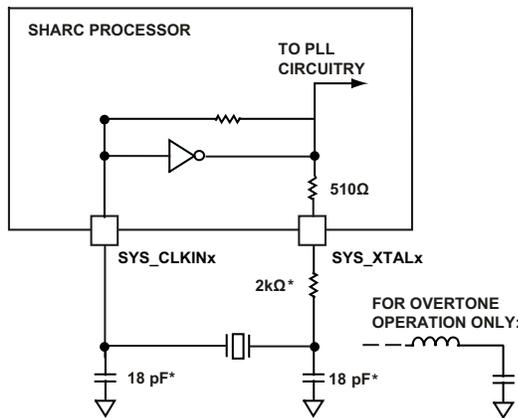
NOTE: VALUES MARKED WITH \* MUST BE CUSTOMIZED, DEPENDING ON THE CRYSTAL AND LAYOUT. ANALYZE CAREFULLY. FOR FREQUENCIES ABOVE 33 MHz, THE SUGGESTED CAPACITOR VALUE OF 18 pF MUST BE TREATED AS A MAXIMUM.
