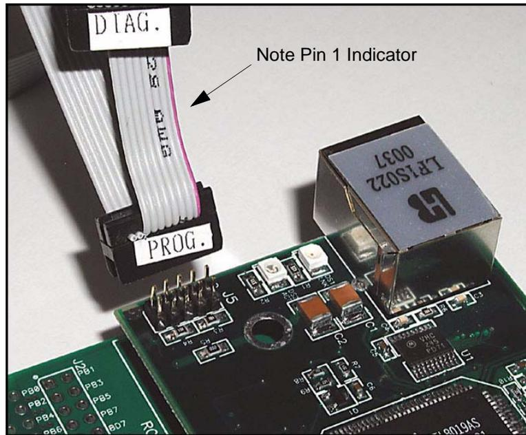
**Figure 3. Attaching Programming Cable to the RCM2100**
