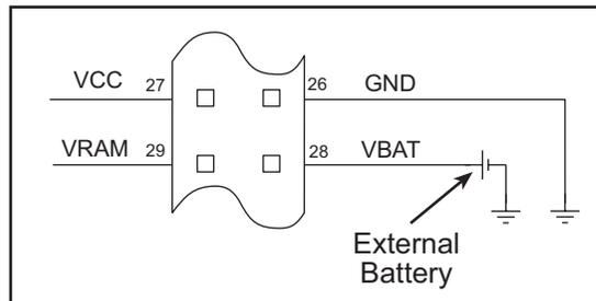
**Figure C-1. External Battery Connections at Header J2**
