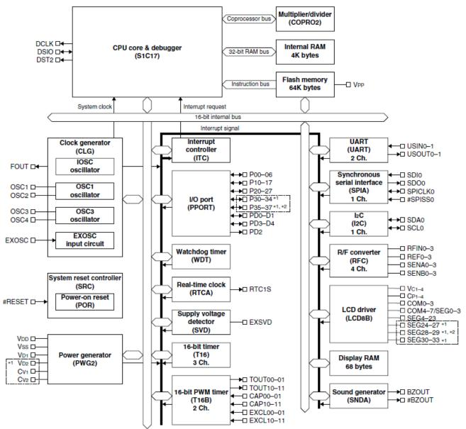
\*1 These pins do not exist in the 64-pin package. \*2 These pins do not exist in the 80-pin package.
