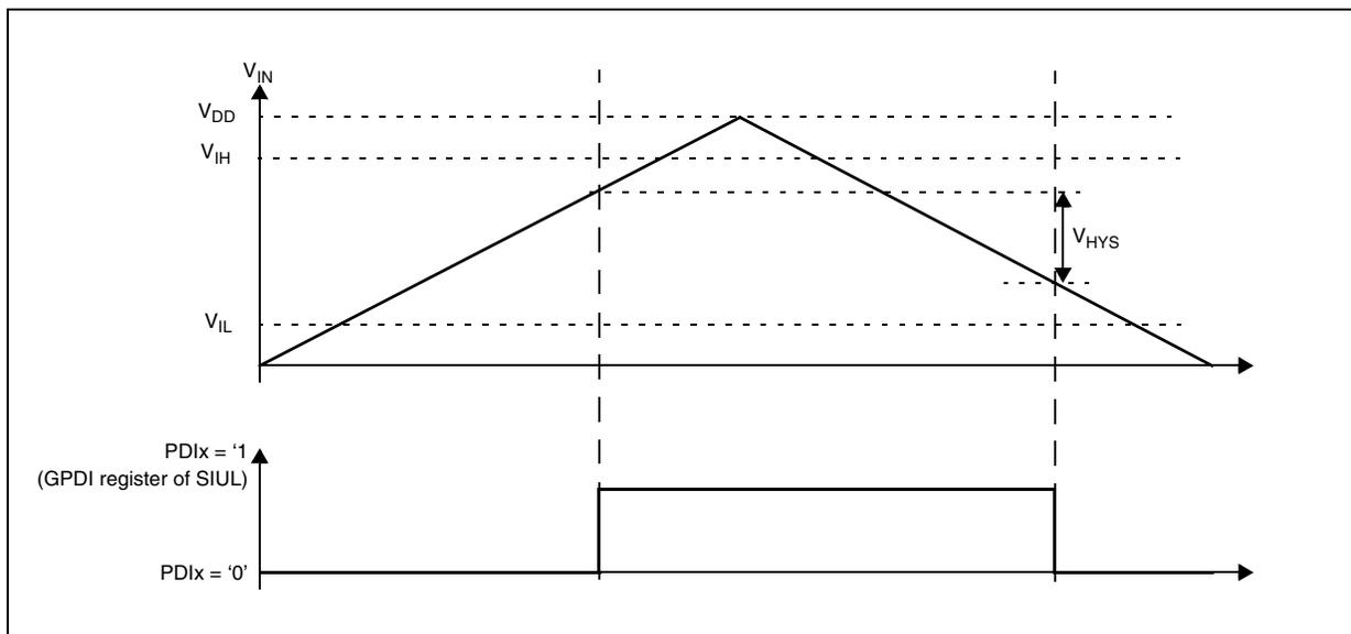
**Figure 5. I/O input DC electrical characteristics definition**
