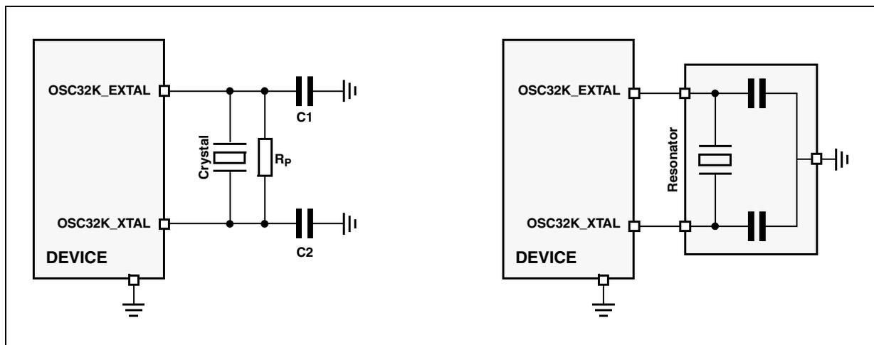
**Figure 14. Crystal oscillator and resonator connection scheme**
