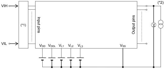
(\*1) Input logic circuit to determine the specified measuring conditions. (\*2) Measured at the specified output pins.
