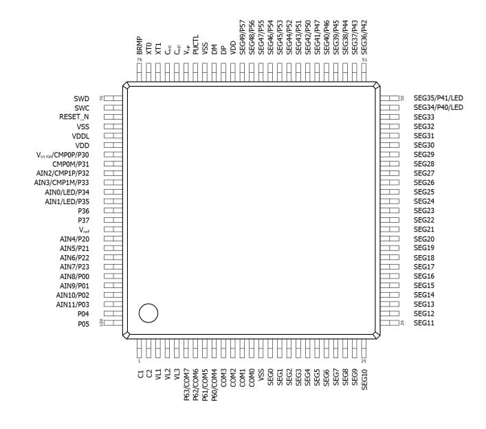
Figure 2. Pin Layout of ML630Q464/Q466
