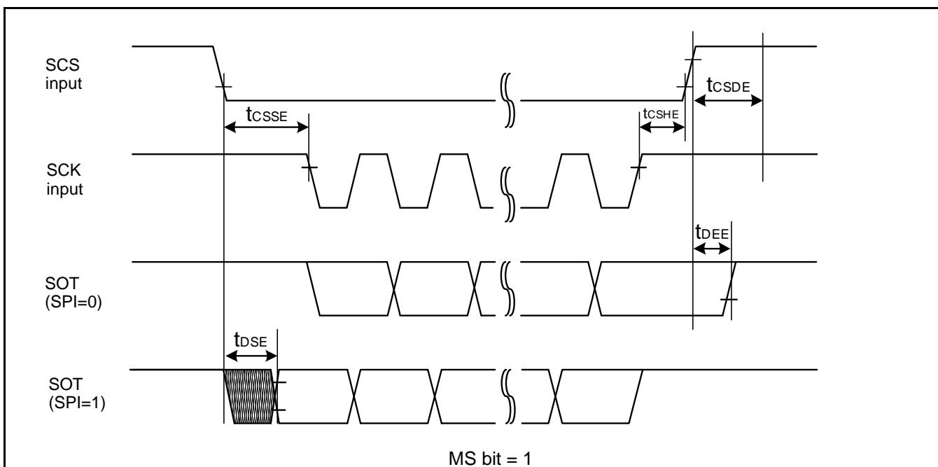
**When Using High-Speed Synchronous Serial Chip Select (SCINV = 1, CSLVL = 1)**
