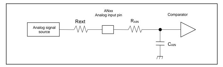
(Equation 1)  $t_S \ge (R_{AIN} + R_{ext}) \times C_{AIN} \times 9$
