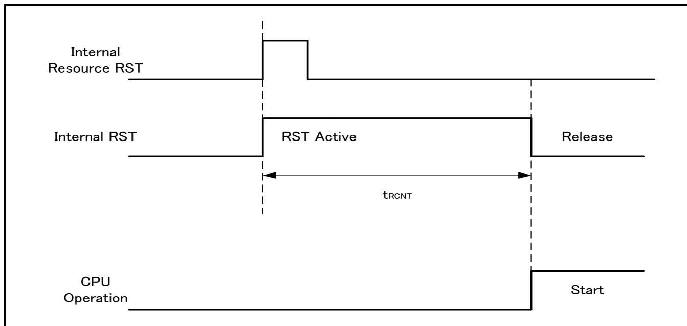
\*: Depending on the low-power consumption mode, the reset issue from the internal resource is not included in the recovery cause.
