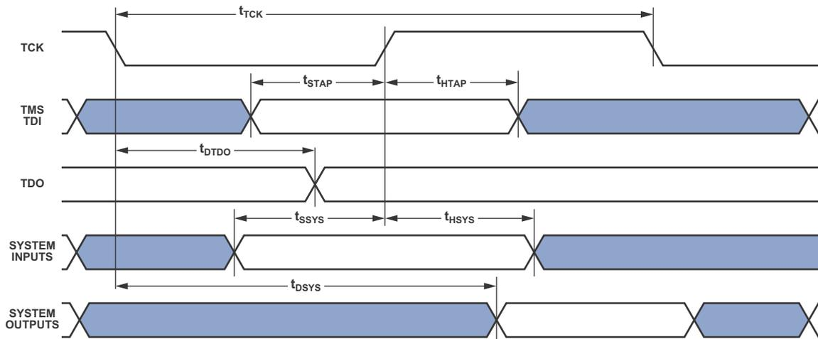
Figure 27. JTAG Test Access Port and Emulation
