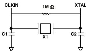
NOTE: C1 AND C2 ARE SPECIFIC TO CRYSTAL SPECIFIED FOR X1. CONTACT CRYSTAL MANUFACTURER FOR DETAILS. CRYSTAL SELECTION MUST COMPLY WITH CLKCFG1-0 = 10 OR = 01.
