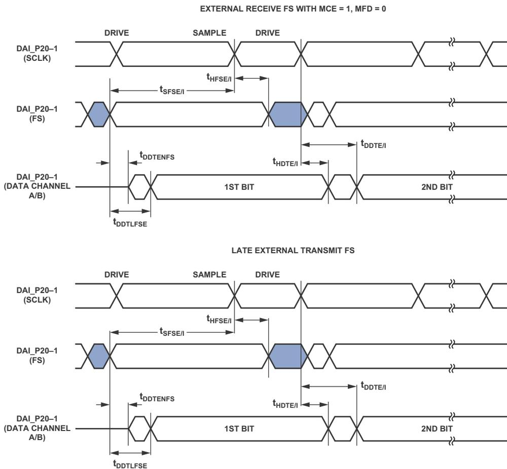
Figure 22. External Late Frame Sync<sup>1</sup>
