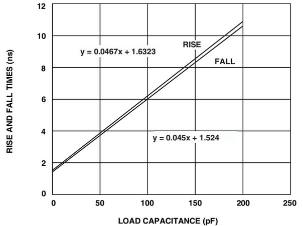
Figure 31. Typical Output Rise Time (20% to 80%,  $V_{DDEXT} = \text{Max}$ )
