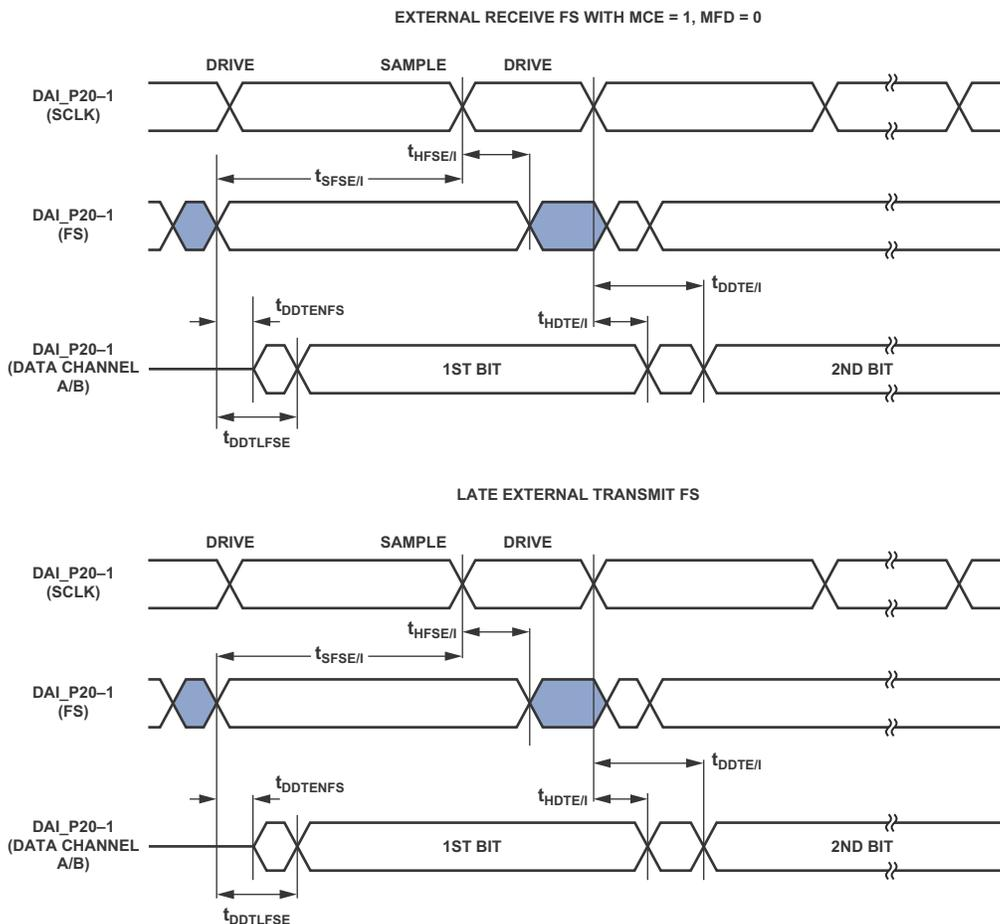
Figure 22. External Late Frame Sync<sup>1</sup>
