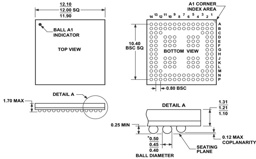
\*COMPLIANT WITH JEDEC STANDARDS MO-205-AE WITH EXCEPTION TO BALL DIAMETER.
