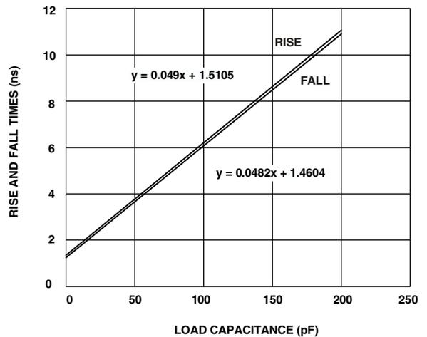
Figure 32. Typical Output Rise/Fall Time (20% to 80%,  $V_{DDEXT} = \text{Min}$ )
