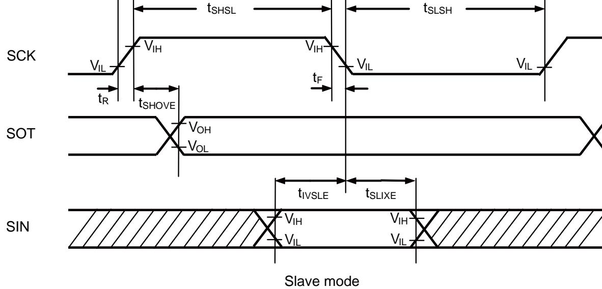
SPI Compatible (SCR: SPI = 1) and Serial Clock Output Signal Detect Level "H" (SMR: SCINV = 0)
