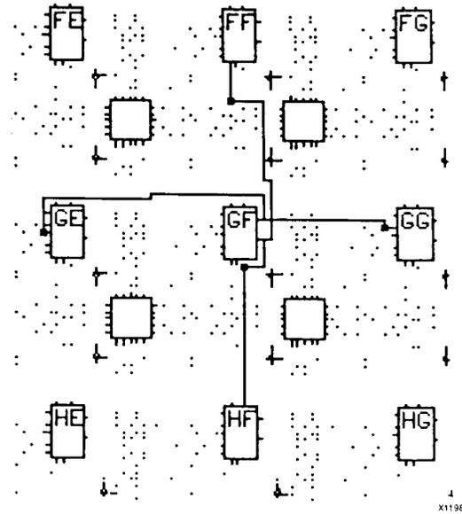
**Figure 12: CLB X and Y Outputs.**
