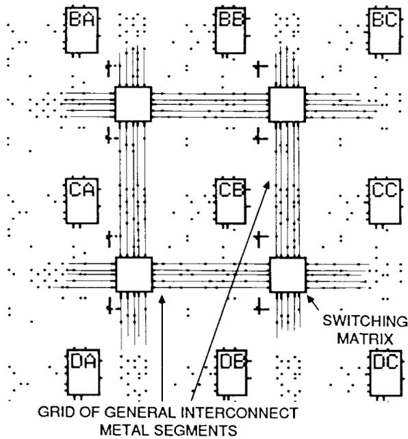
**Figure 10: FPGA General-Purpose Interconnect.**
