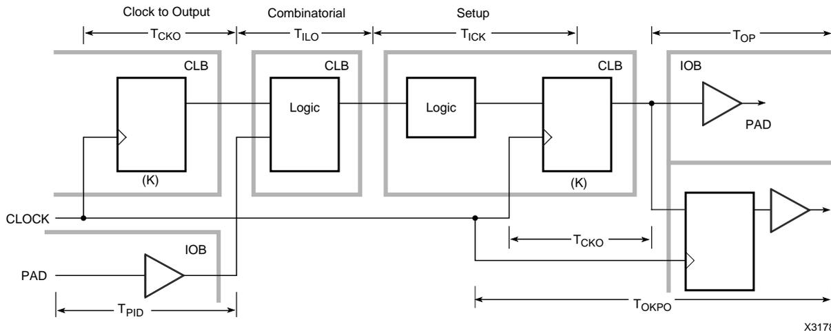
**Figure 31: Primary Block Speed Factors.** Actual timing is a function of various block factors combined with routing factors. Overall performance can be evaluated with the timing calculator or by an optional simulation.
