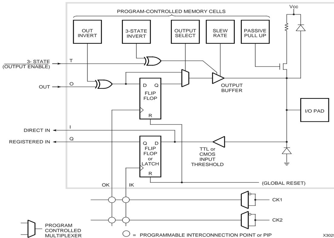
**Figure 4: Input/Output Block.**
