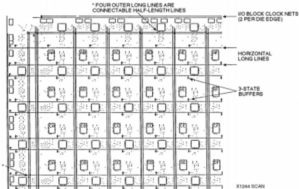
**Figure 15: Programmable Interconnection of Longlines.** This is provided at the edges of the routing area. Three-state buffers allow the use of horizontal Longlines to form on-chip wired AND and multiplexed buses. The left two non-clock vertical Longlines per column (except XC3020A) and the outer perimeter Longlines may be programmed as connectable half-length lines.
