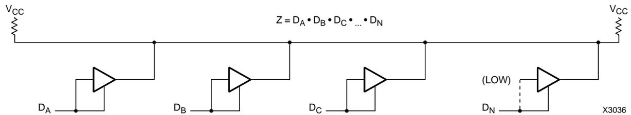
**Figure 16: 3-State Buffers Implement a Wired-AND Function.** When all the buffer 3-state lines are High, (high impedance), the pull-up resistor(s) provide the High output. The buffer inputs are driven by the control signals or a Low.
