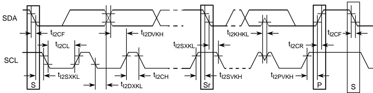
Figure 47. I<sup>2</sup>C Bus AC Timing Diagram
