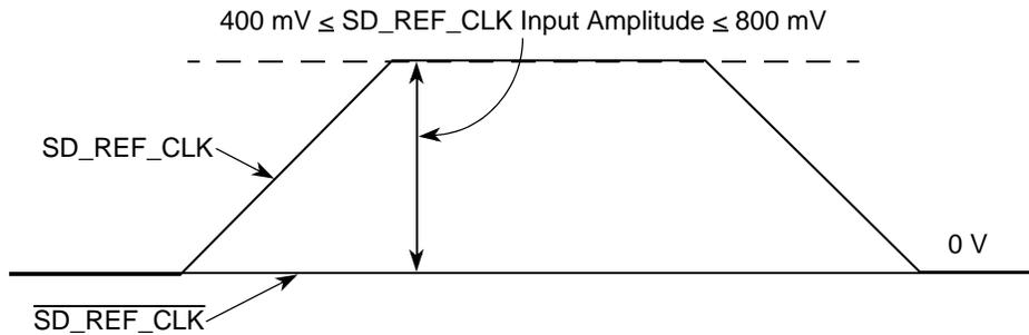
**Figure 26. Single-Ended Reference Clock Input DC Requirements**
