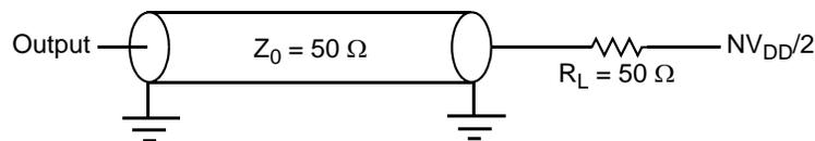
**Figure 51. Timers AC Test Load**
