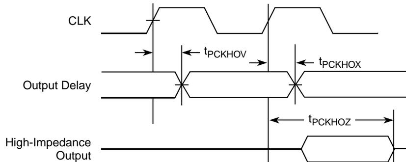
**Figure 50. PCI Output AC Timing Measurement Condition**
