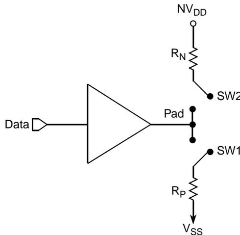
**Figure 60. Driver Impedance Measurement**
