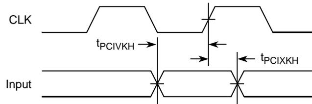
**Figure 49. PCI Input AC Timing Measurement Conditions**
