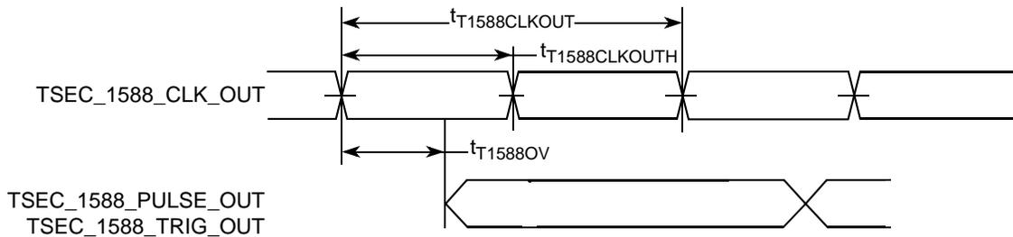
**Note:** The output delay is count starting rising edge if  $t_{T1588CLKOUT}$  is non-inverting. Otherwise, it is count starting falling edge.
