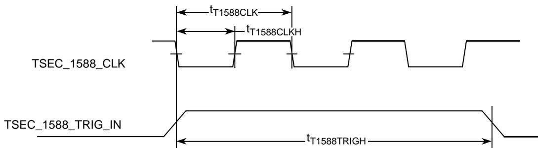
Figure 20. eTSEC IEEE 1588 Input AC Timing
