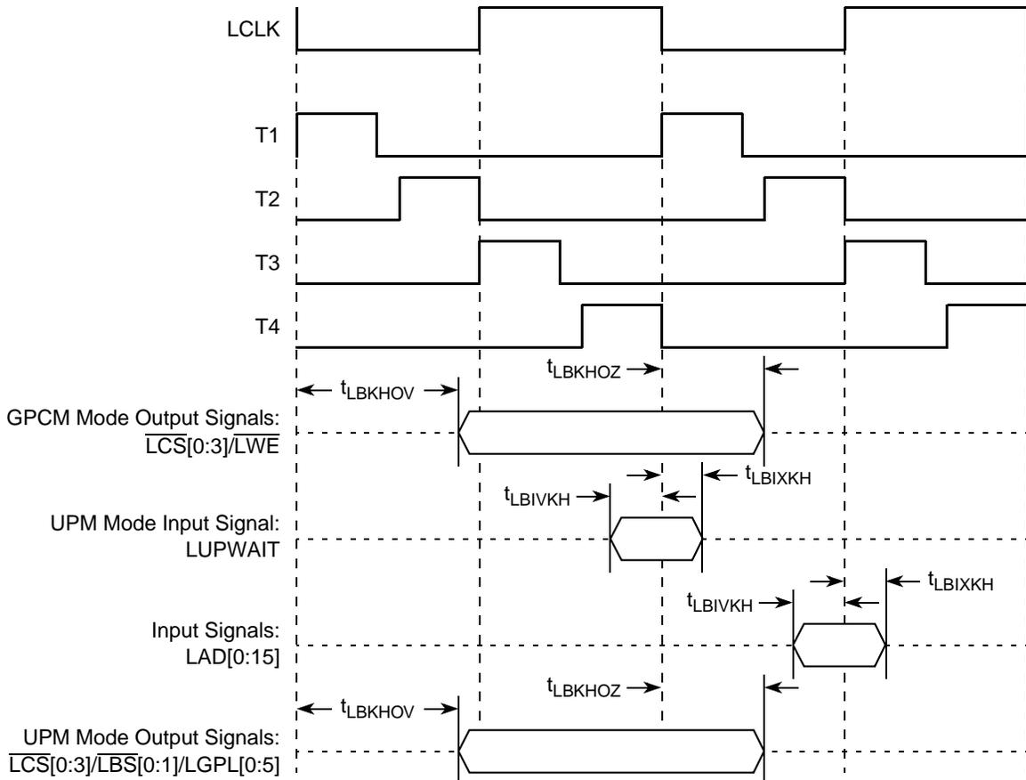
**Figure 39. Local Bus Signals, GPCM/UPM Signals for LCRR[CLKDIV] = 4**
