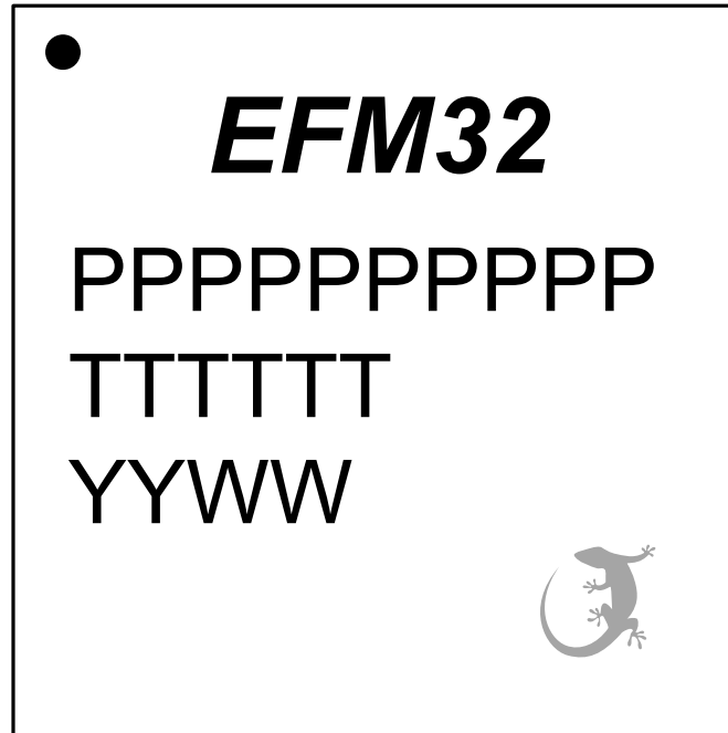
Figure 8.3. QFN48 Package Marking
