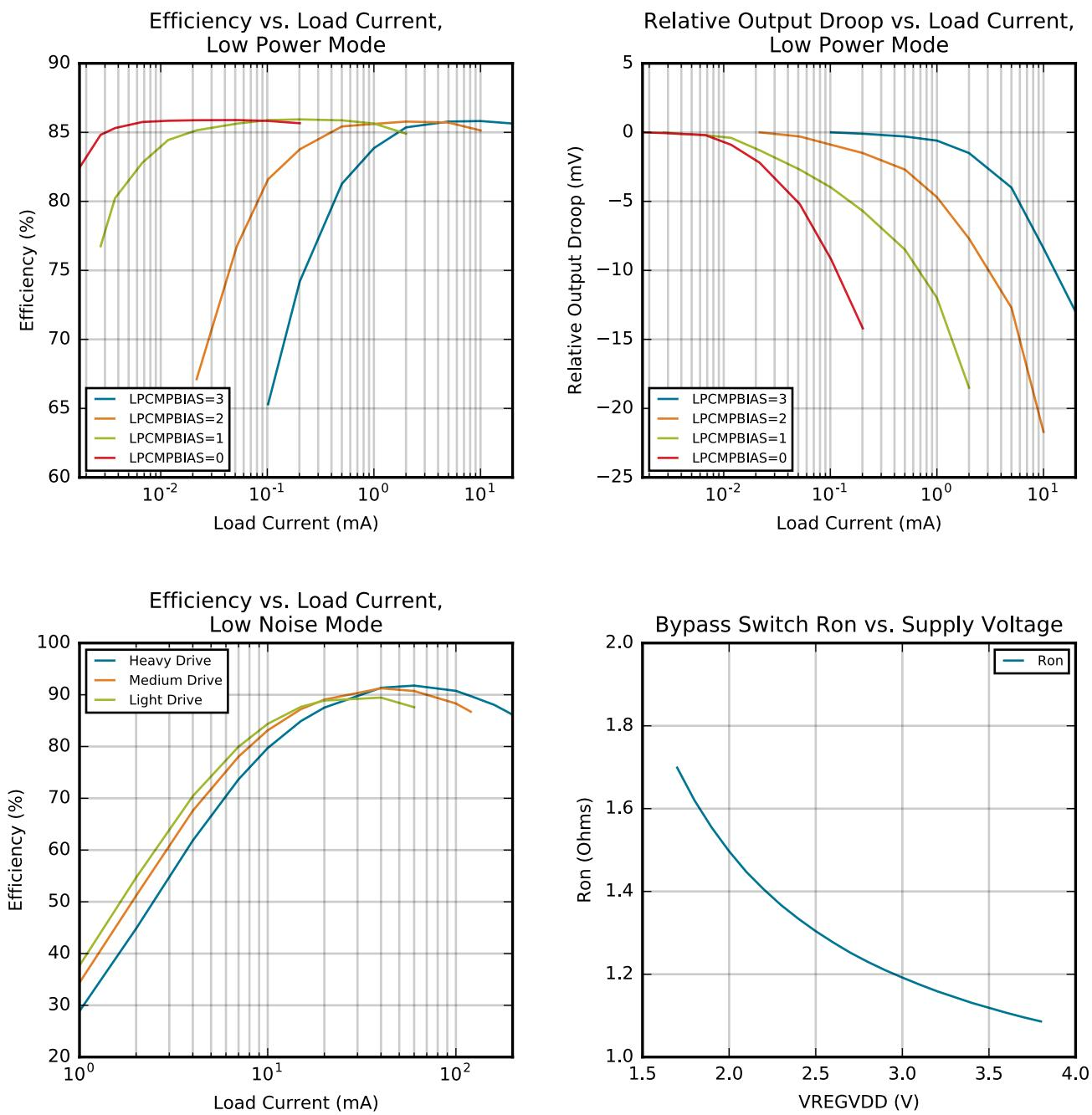
Figure 4.8. DC-DC Converter Typical Performance Characteristics
