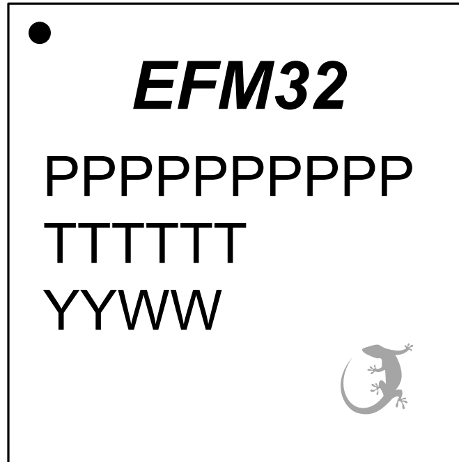
Figure 8.3. QFN48 Package Marking
