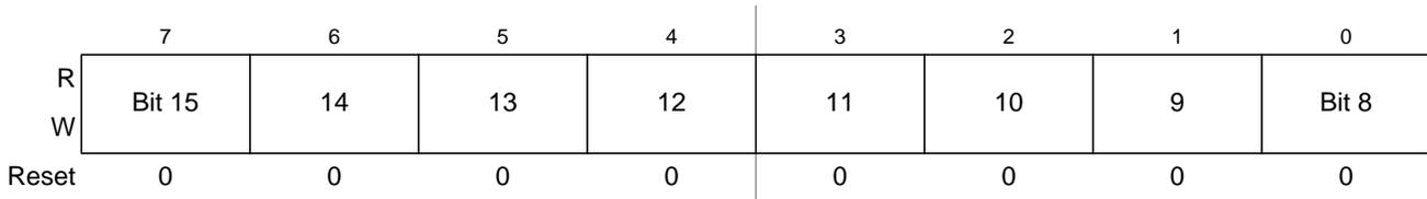
Figure 16-10. TPM Counter Modulo Register High (TPMxMODH)
