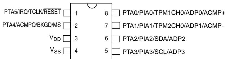
Figure 2-4. 8-Pin SOIC
