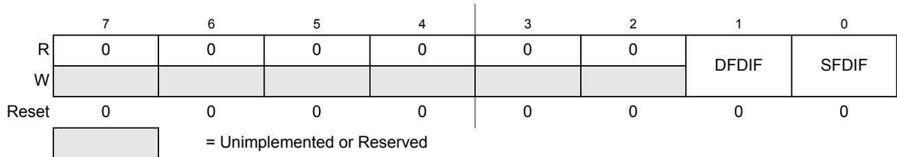
Figure 30-12. Flash Error Status Register (FERSTAT)
