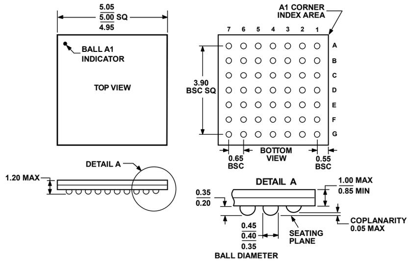
Figure 101. 49-Ball Chip Scale Package Ball Grid Array [CSP\_BGA]
