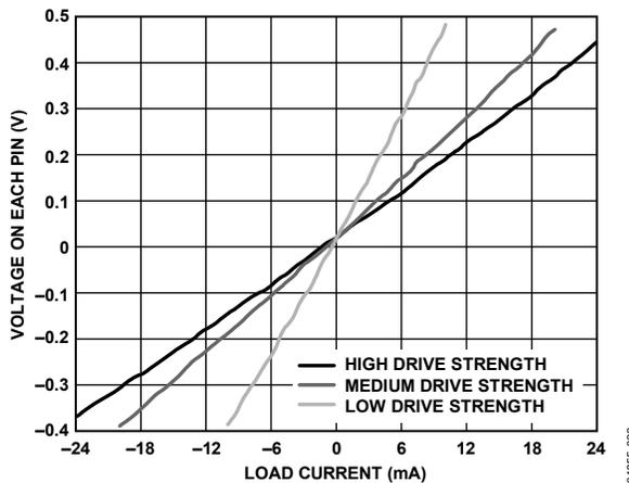
Figure 74. Programmable Strength for Low Level (Typical Values)
