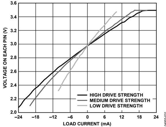
Figure 73. Programmable Strength for High Level (Typical Values)
