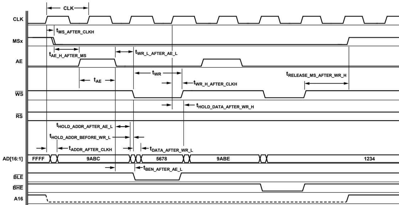
Figure 12. External Memory Write Cycle (See Table 78)
