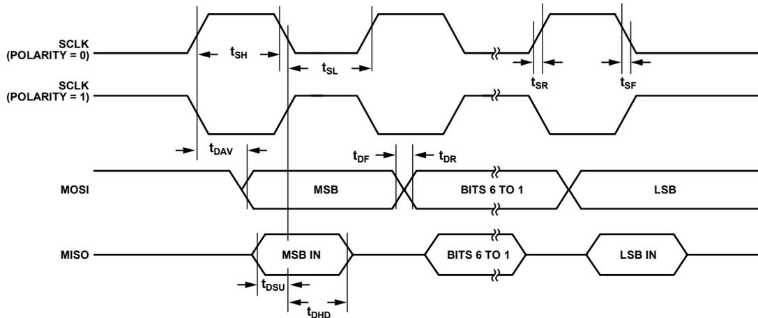
Figure 15. SPI Master Mode Timing (Phase Mode = 1)
