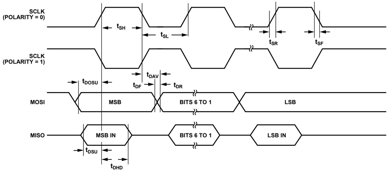
Figure 16. SPI Master Mode Timing (Phase Mode = 0)
