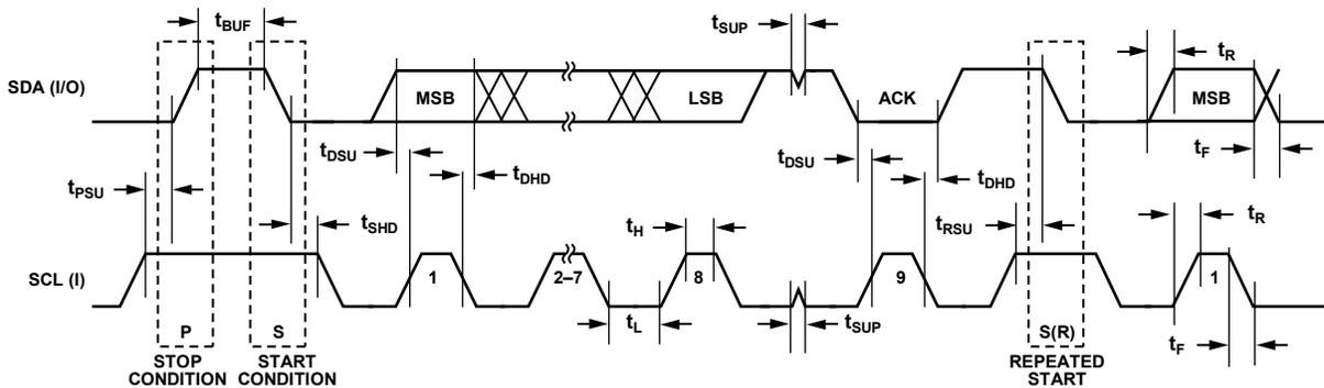
Figure 14. I<sup>2</sup>C Compatible Interface Timing
