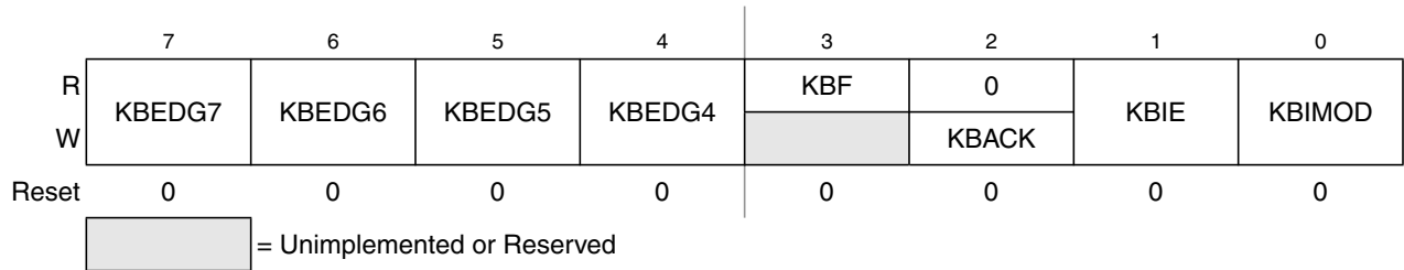
Figure 9-3. KBI x Status and Control Register (KBIXSC)
