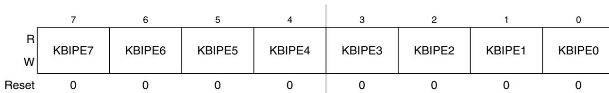
Figure 9-4. KBI x Pin Enable Register (KBIXPE)
