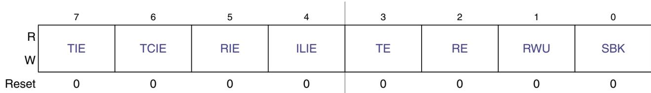
Figure 12-6. SCI Control Register 2 (SCI1C2)
