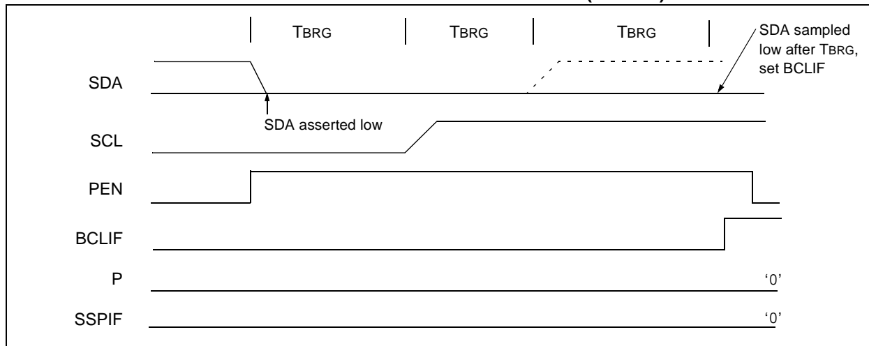
FIGURE 13-26: BUS COLLISION DURING A STOP CONDITION (CASE 1)
