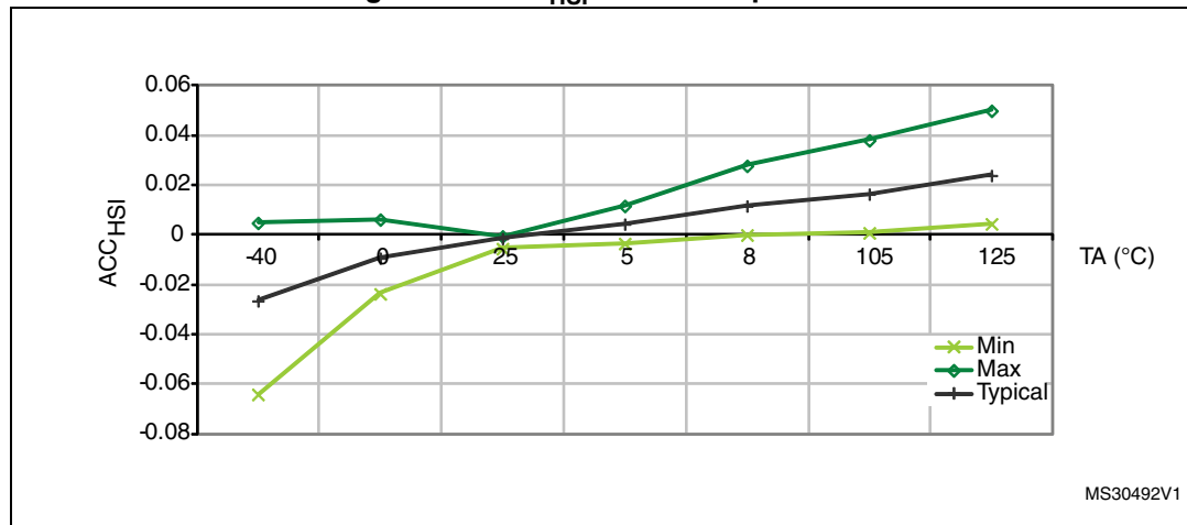
Figure 31. ACC_{HSI} versus temperature
