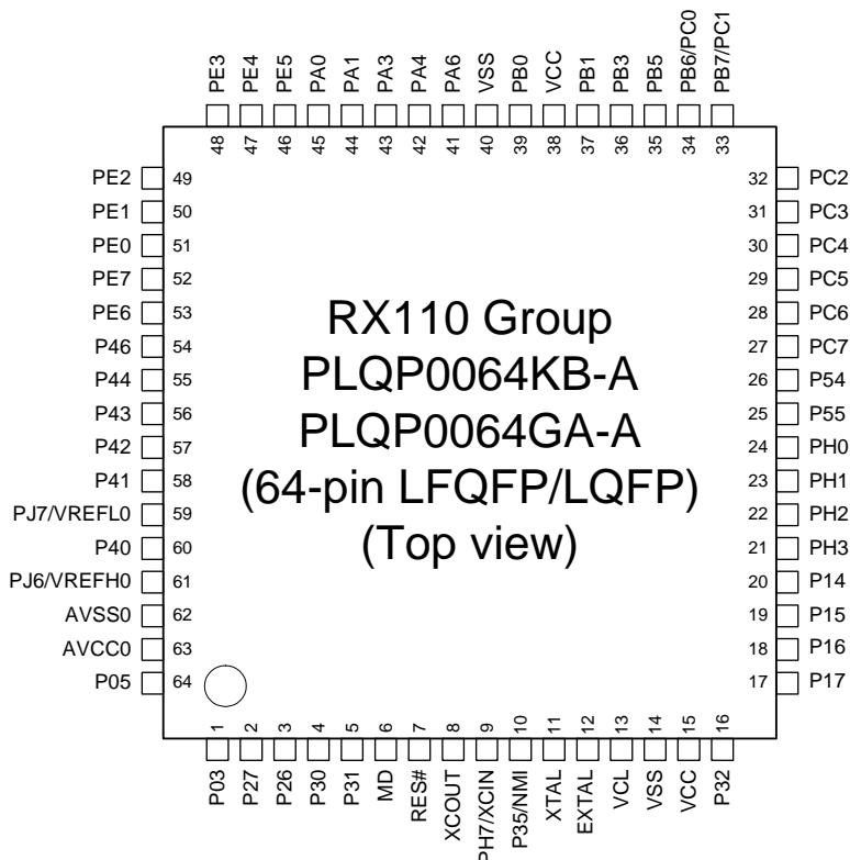
Note: This figure indicates the power supply pins and I/O ports.
