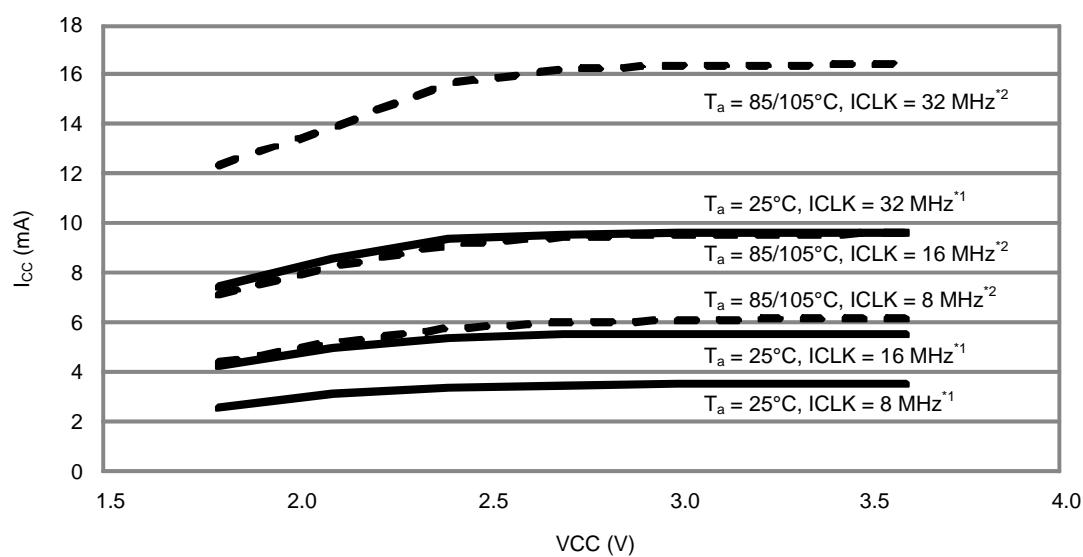
Note 1. All peripheral operation is normal. Average value of the tested middle samples during product evaluation.
