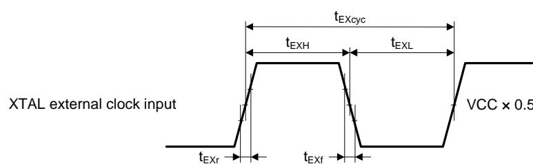
**Figure 5.18 XTAL External Clock Input Timing**
