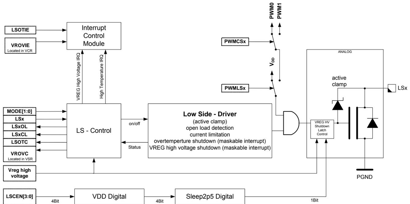
Figure 21. Low Side Drivers - Block Diagram
