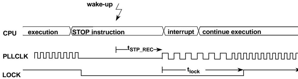
Figure 88. Stop Mode Using PLLCLK as Bus Clock
