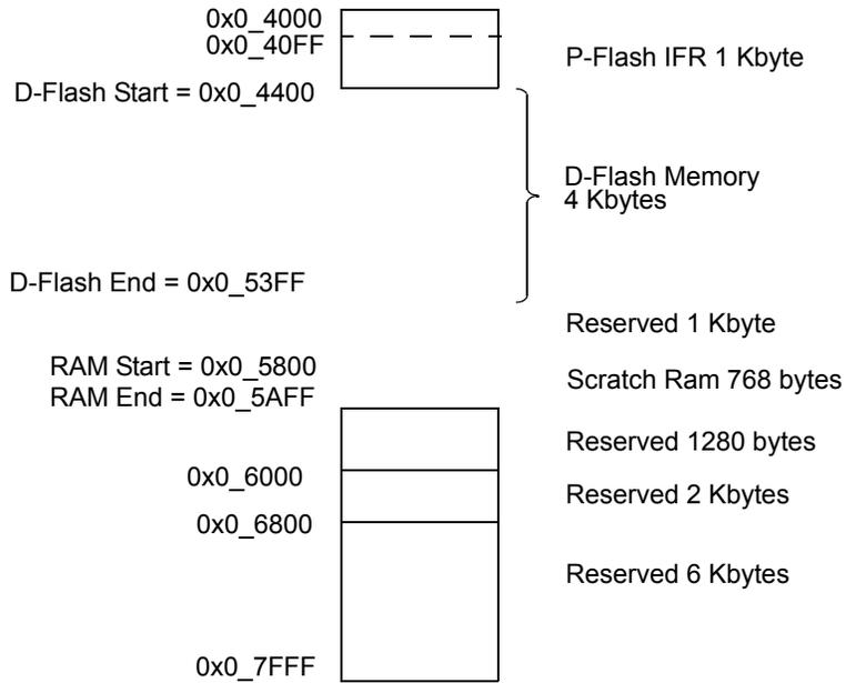
**Figure 105. D-Flash and Memory Controller Resource Memory Map**
