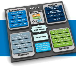
Based on the powerful ARM® Cortex®-M4 processor, the Atmel® | SMART SAM4S series extends the Atmel® ARM Cortex-Mbased microcontroller (MCU) portfolio to offer:
