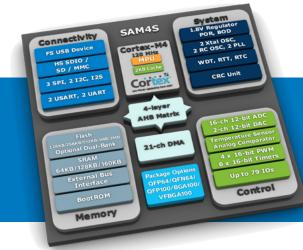
Based on the powerful ARM® Cortex®-M4 processor, the Atmel® | SMART SAM4S series extends the Atmel® ARM Cortex-M-based microcontroller (MCU) portfolio to offer:
