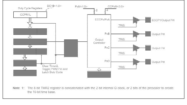
Note:The TRIS register value for each PWM output must be configured appropriately.Any pin not used by an Enhanced PWM mode is available for alternate pin functions.
