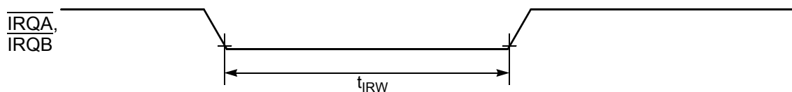
Figure 10-6 External Interrupt Timing (Negative Edge-Sensitive)
