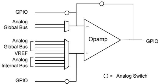
The opamp is uncommitted and can be configured as a gain stage or voltage follower, or output buffer on external or internal signals.
