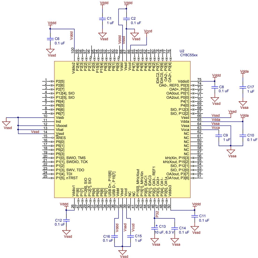
**Note** The two Vccd pins must be connected together with as short a trace as possible. A trace under the device is recommended, as shown in Figure 2-6 on page 10.
