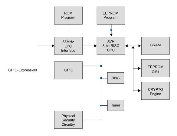
The TPM includes a hardware random number generator, including a FIPS-approved Pseudo Random Number Generator that is used for key generation and TCG protocol functions. The RNG is also available to the system to generate random numbers that may be needed during normal operation.
