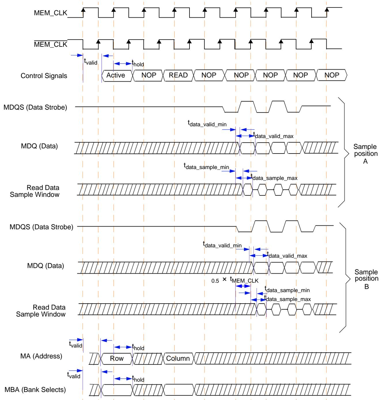
Sample position A: data are sampled on the expected edge of MEM\_CLK, the MDQS signal indicate the valid data
