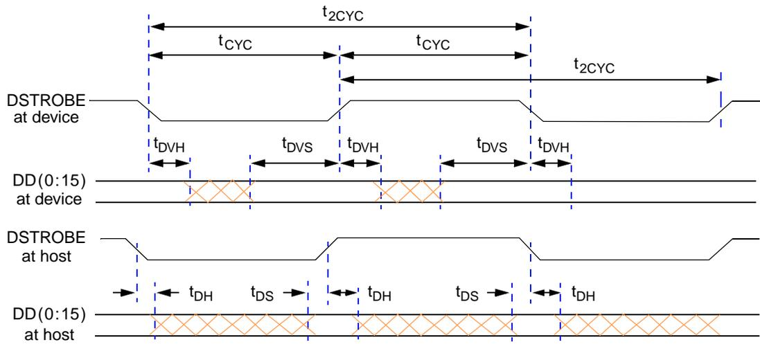
**Figure 17. Timing Diagram—Sustained Ultra DMA Data In Burst**
