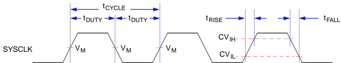
**Figure 2. Timing Diagram—SYS\_XTAL\_IN**
