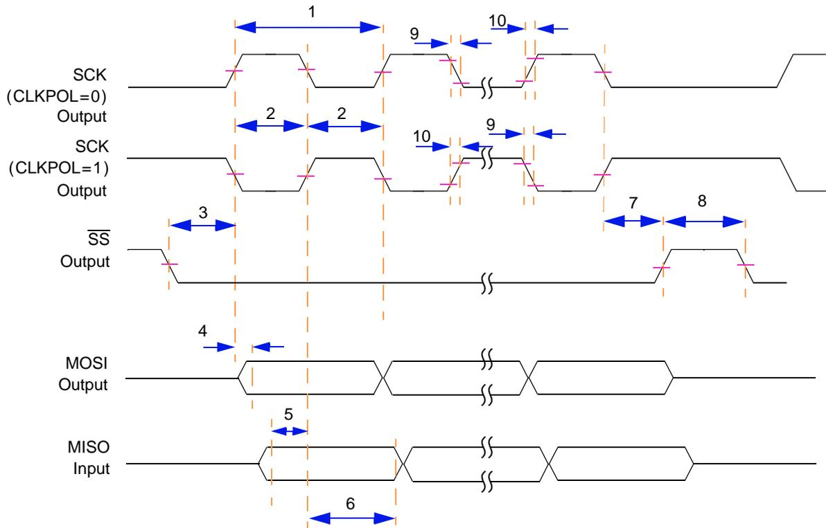
**Figure 43. Timing Diagram — SPI Master Mode, Format 1 (CPHA = 1)**
