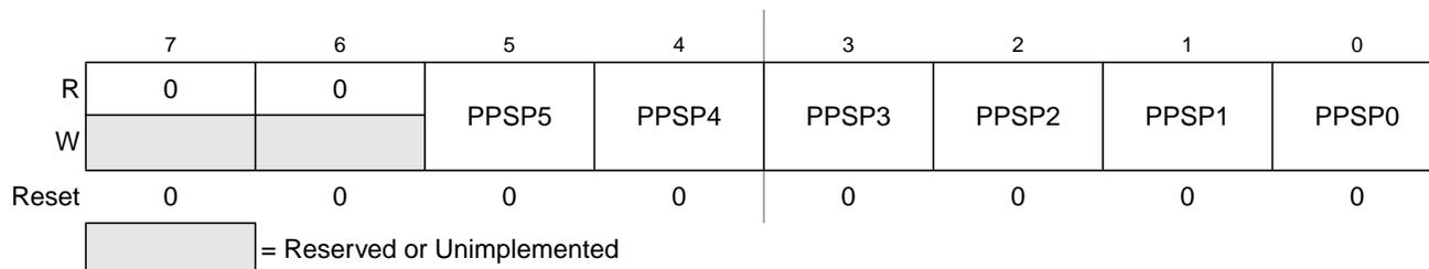
**Figure 3-22. Port P Polarity Select Register (PPSP)**
