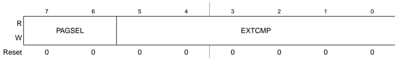
Figure 16-9. Debug Comparator C Extended Register (DBGCCX)
