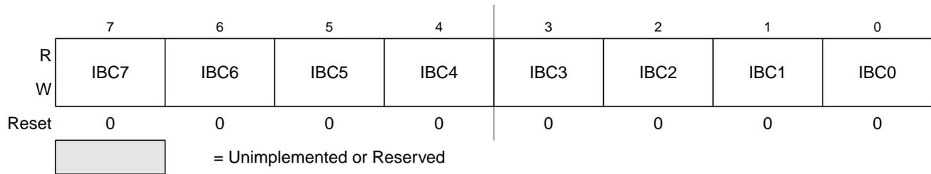
**Figure 10-3. IIC Bus Frequency Divider Register (IBFD)**
