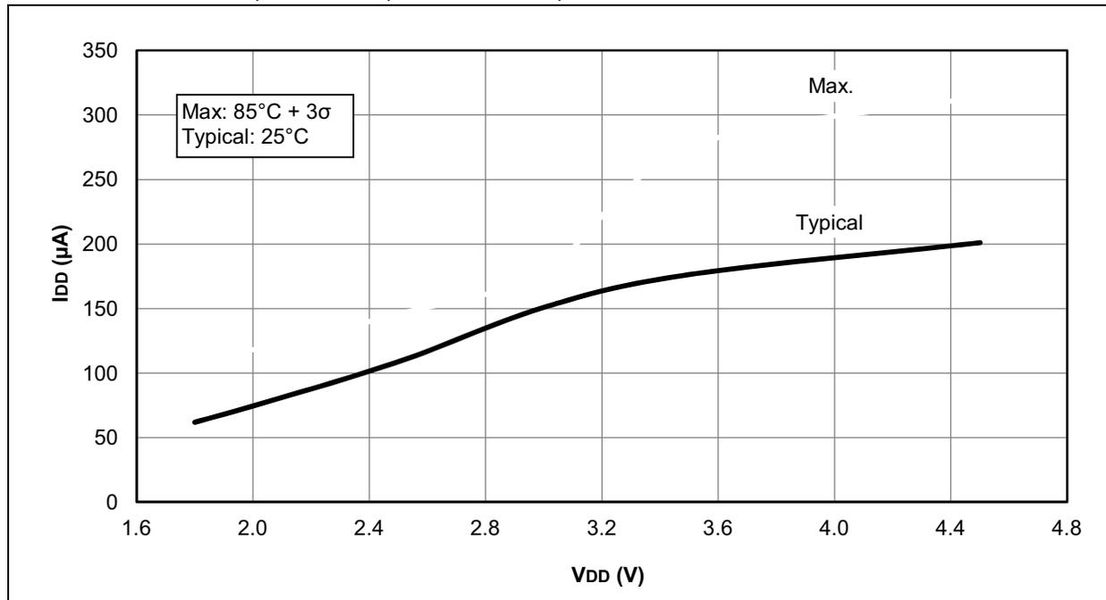
FIGURE 23-10:  $I_{DD}$ , LFINTOSC,  $F_{osc} = 31$  kHz, PIC16F753 ONLY
