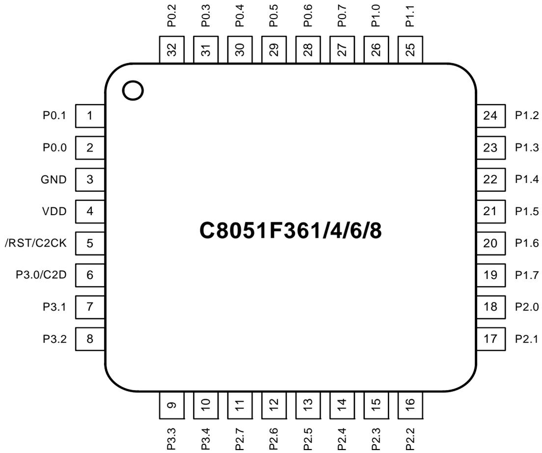
Figure 4.3. LQFP-32 Pinout Diagram (Top View)
