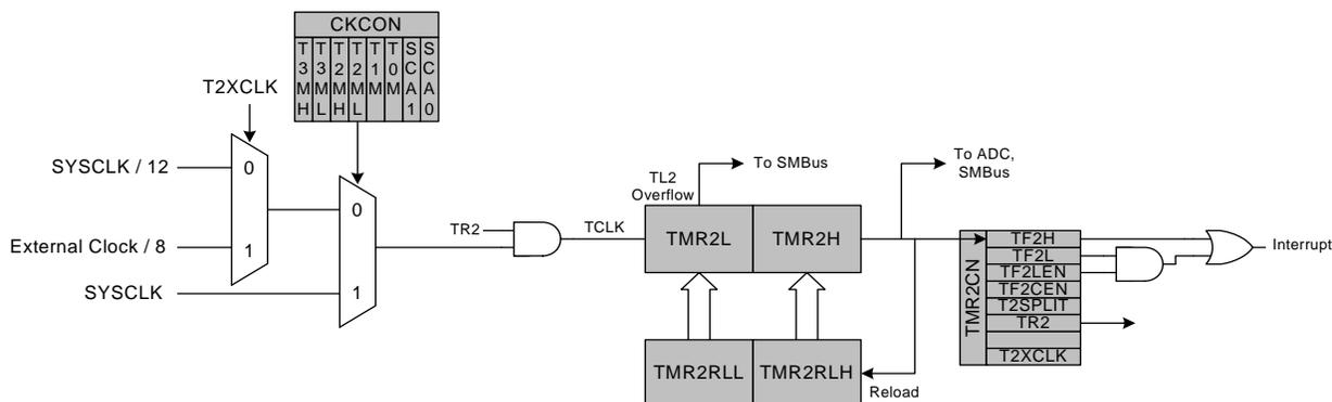
Figure 21.4. Timer 2 16-Bit Mode Block Diagram
