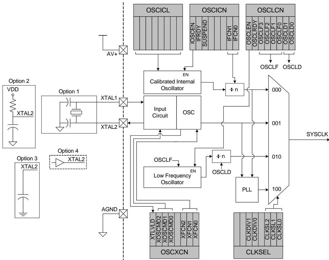
**Figure 16.1. Oscillator Diagram**
