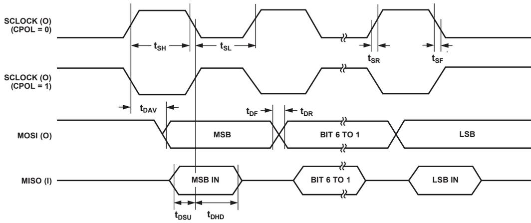
Figure 10. SPI Master Mode Timing (CPHA = 1)
