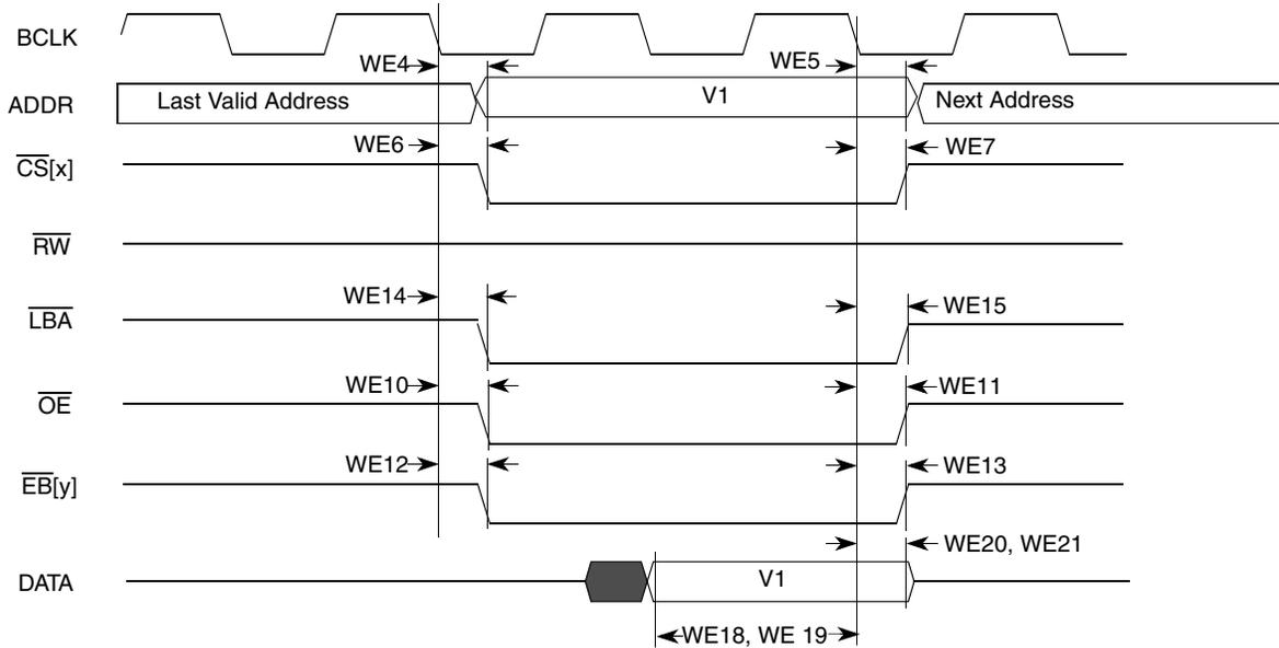
**Figure 16. Synchronous Memory Timing Diagram for Read Access—WSC = 1**
