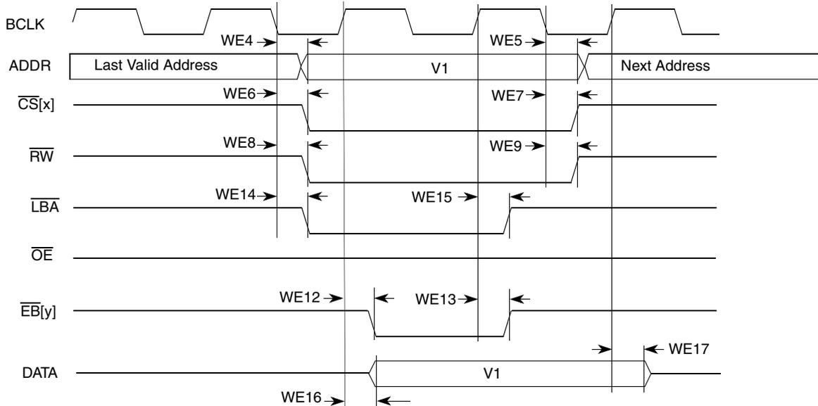
**Figure 17. Synchronous Memory Timing Diagram for Write Access—
