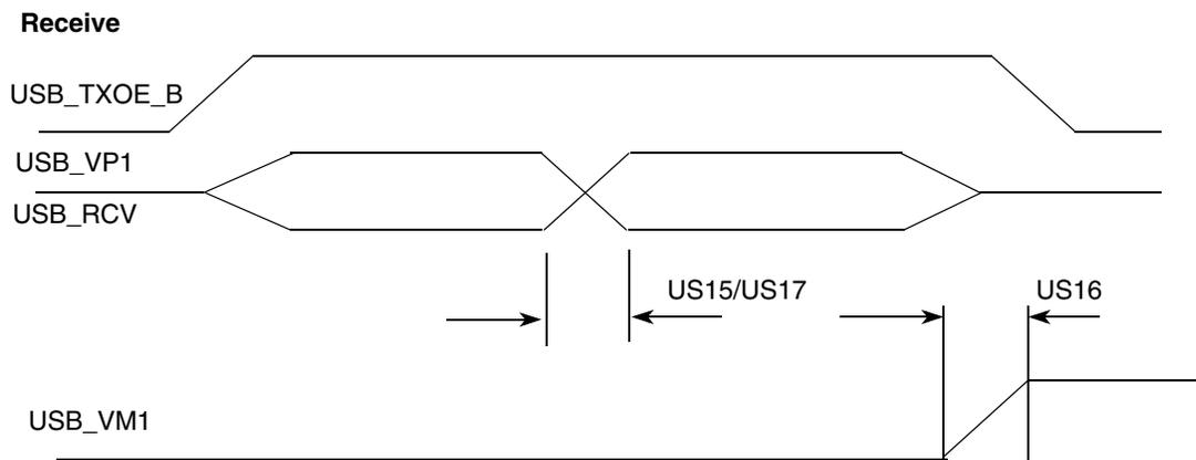
**Figure 103. USB Receive Waveform in DAT\_SE0 Unidirectional Mode**
