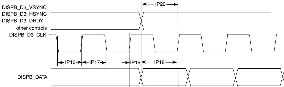
**Figure 50. Synchronous Display Interface Timing Diagram—Access Level**
