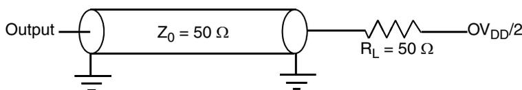
**Figure 36. I<sup>2</sup>C AC Test Load**
