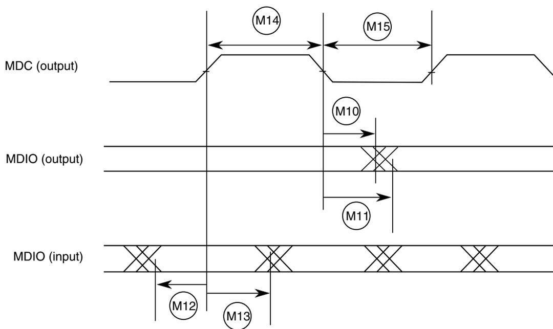
Figure 44. MII serial management channel timing diagram
