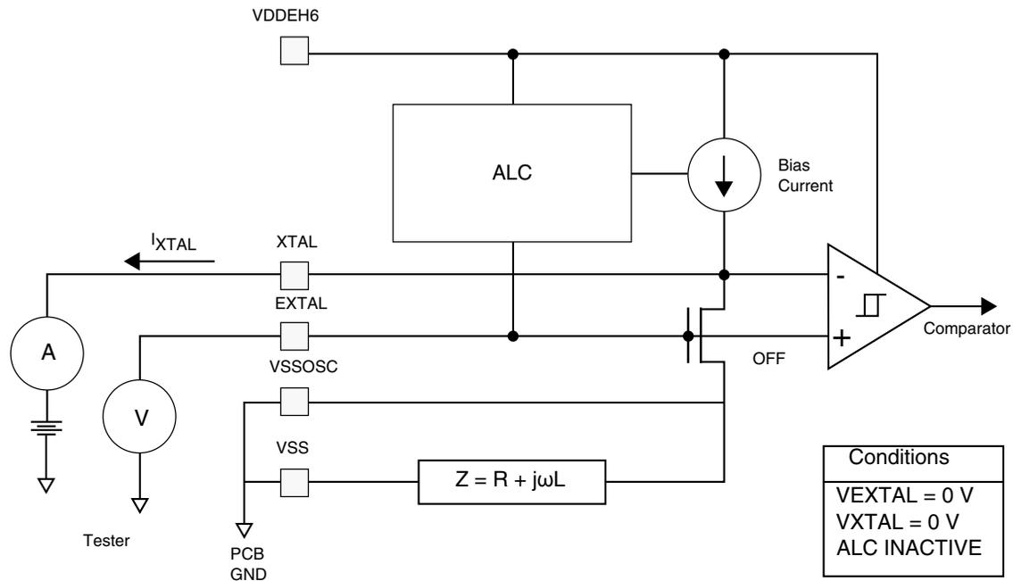
**Figure 7. Test circuit****Table 16. Internal RC (IRC) oscillator electrical specifications**
