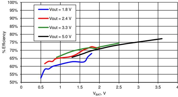
**Figure 11-12. Efficiency vs  $V_{BAT}$ ,  $L_{BOOST} = 10 \mu H$  [33]**
