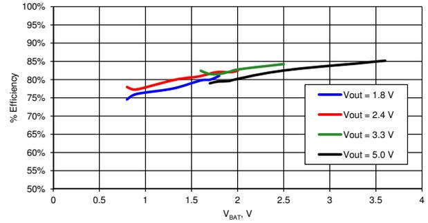
**Figure 11-13. Efficiency vs  $V_{BAT}$ ,  $L_{BOOST} = 22 \mu H$  [33]**
