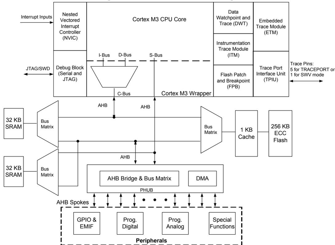
The Cortex-M3 CPU subsystem includes these features:
