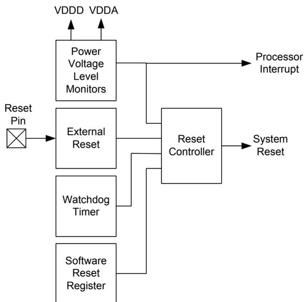
The term **system reset** indicates that the processor as well as analog and digital peripherals and registers are reset.
