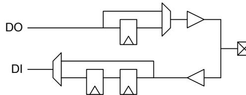
**Figure 7-12. I/O Pin Output Connectivity**
