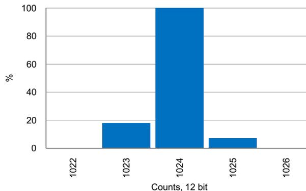
**Figure 11-41. SAR ADC Noise Histogram, 1 msp, External Reference**
