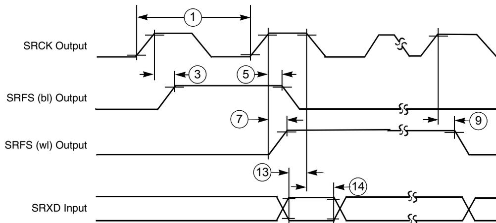
**Figure 51. SSI Receiver Internal Clock Timing Diagram**
